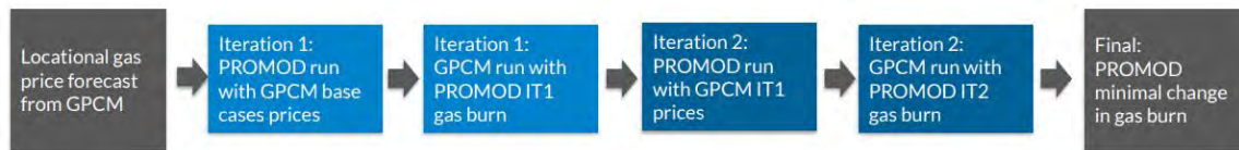
Figure 2.13: GPCM iterative process
