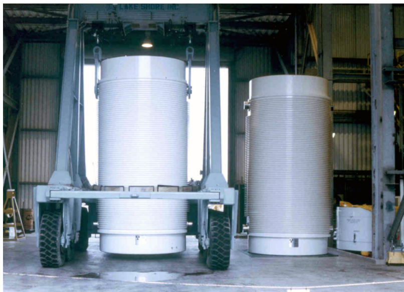
Loaded spent fuel storage cask on transporter is moved from the fuel handling building at the Surry Power Station in Surry, VA.
