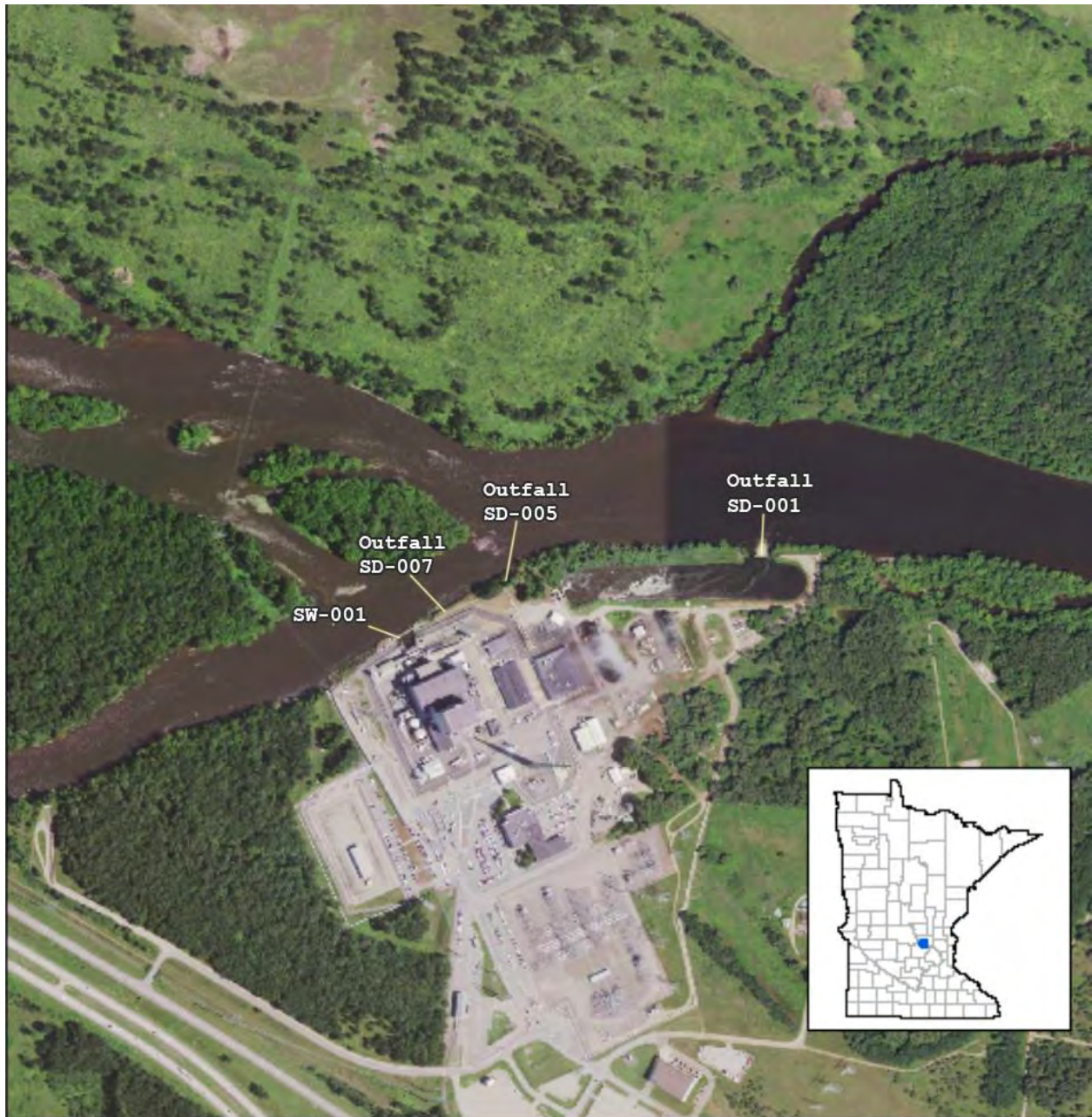
Figure 3-3 Monticello Nuclear Generating Plant External National Pollutant Discharge Elimination System Monitoring Locations. Adapted from: Xcel 2023-TN9084, Fig 3.6-3.
