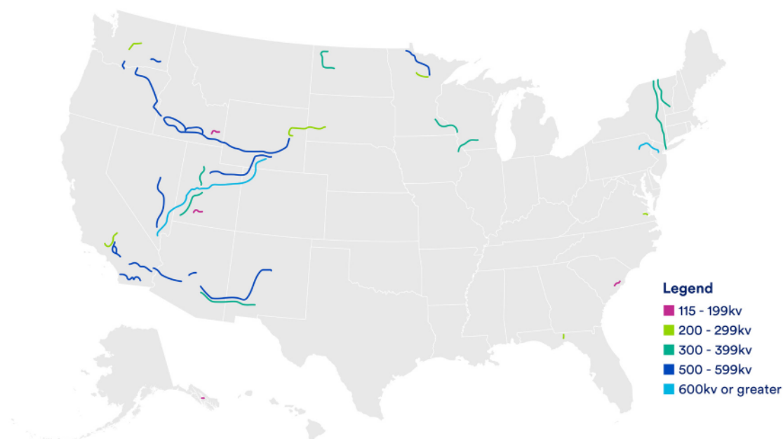
Figure 1: Map of the 33 Completed Lines in the EIS Lines Dataset, by Voltage Class. (4 of the original 37 lines were canceled and therefore not included)
