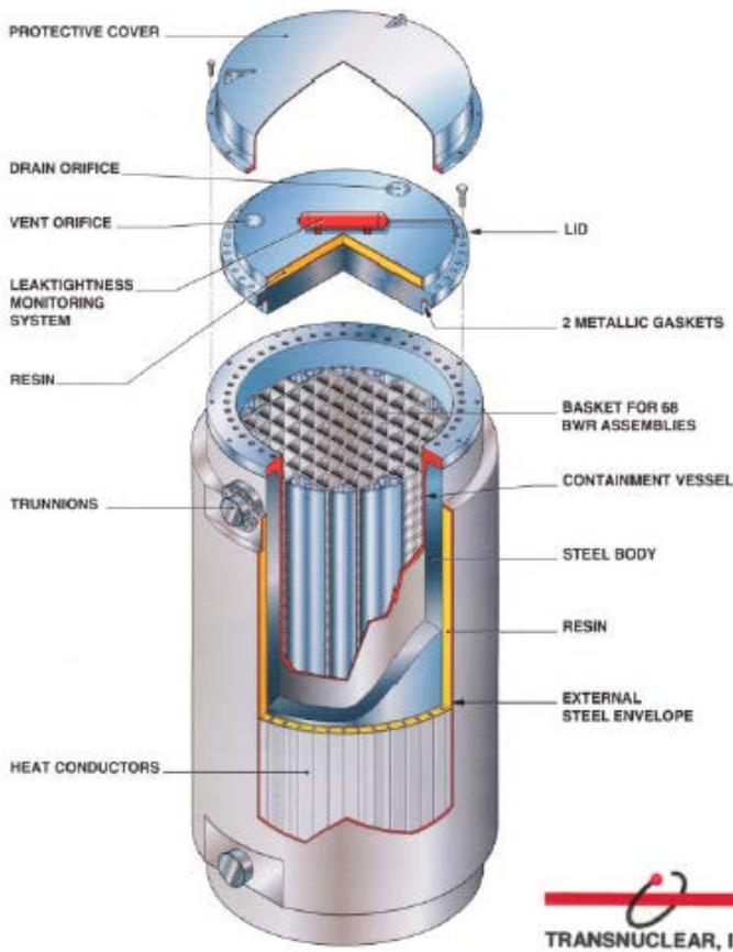
The thick metal cask body provides physical protection and radiation shielding for the spent fuel. Cask bodies are either all steel or a steel and lead combination. The casks use a bolted closure consisting of a single lid with dual metallic seals. The annulus between the seals is pressurized and connected to a system that monitors the annulus for loss of pressure. The casks are stored outdoors on a concrete pad.
