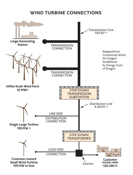
wire the system and have the installation inspected by a state certified electrical inspector to make sure that all of the relevant safety rules have been followed. You should also consult your electrical power supplier to evaluate their distribution system for the extra load before installation and perform a stray voltage investigation on your livestock operation before and after the installation of a wind turbine.
