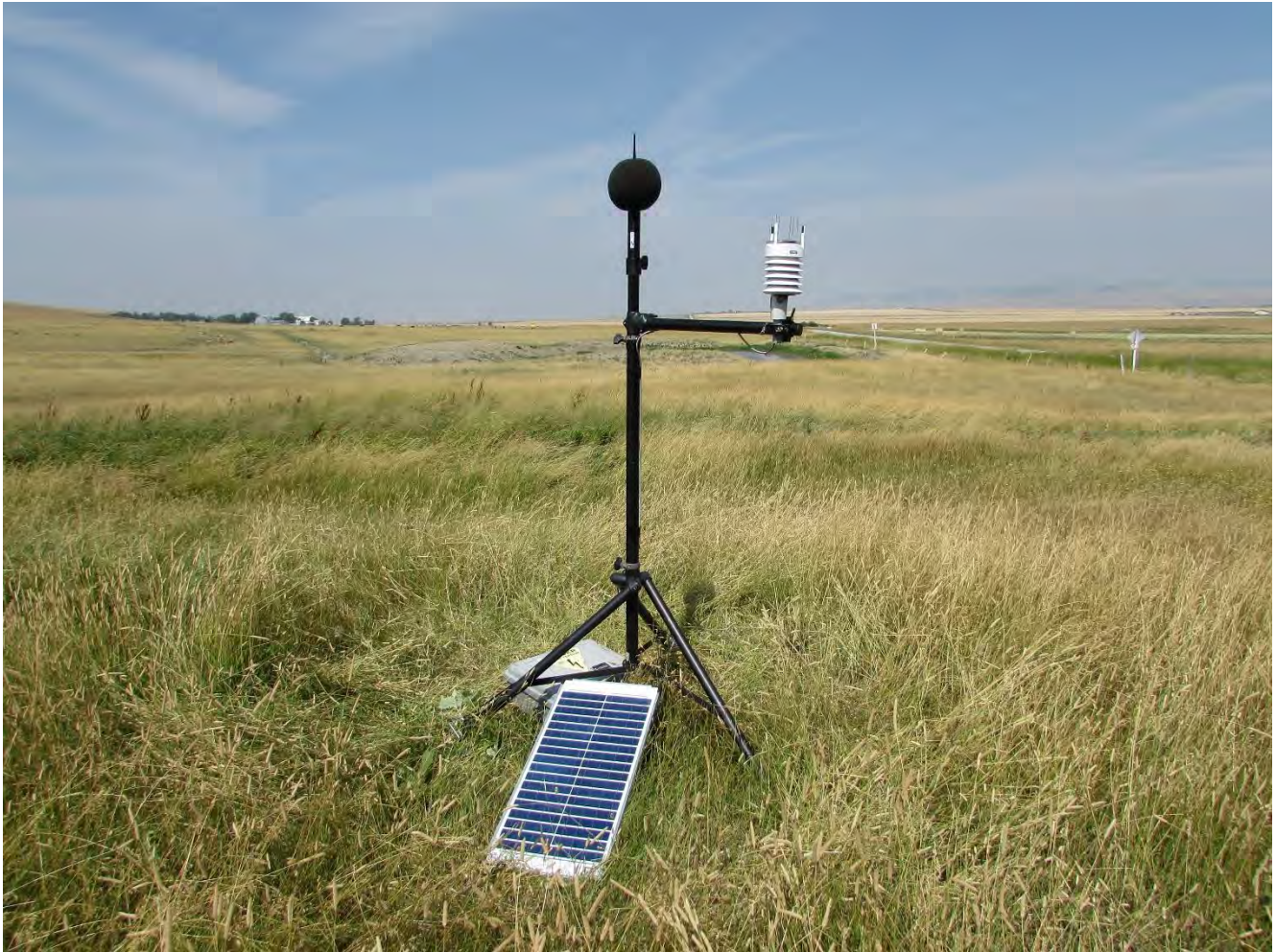
In-situ set-up of Sound Measurement Equipment
