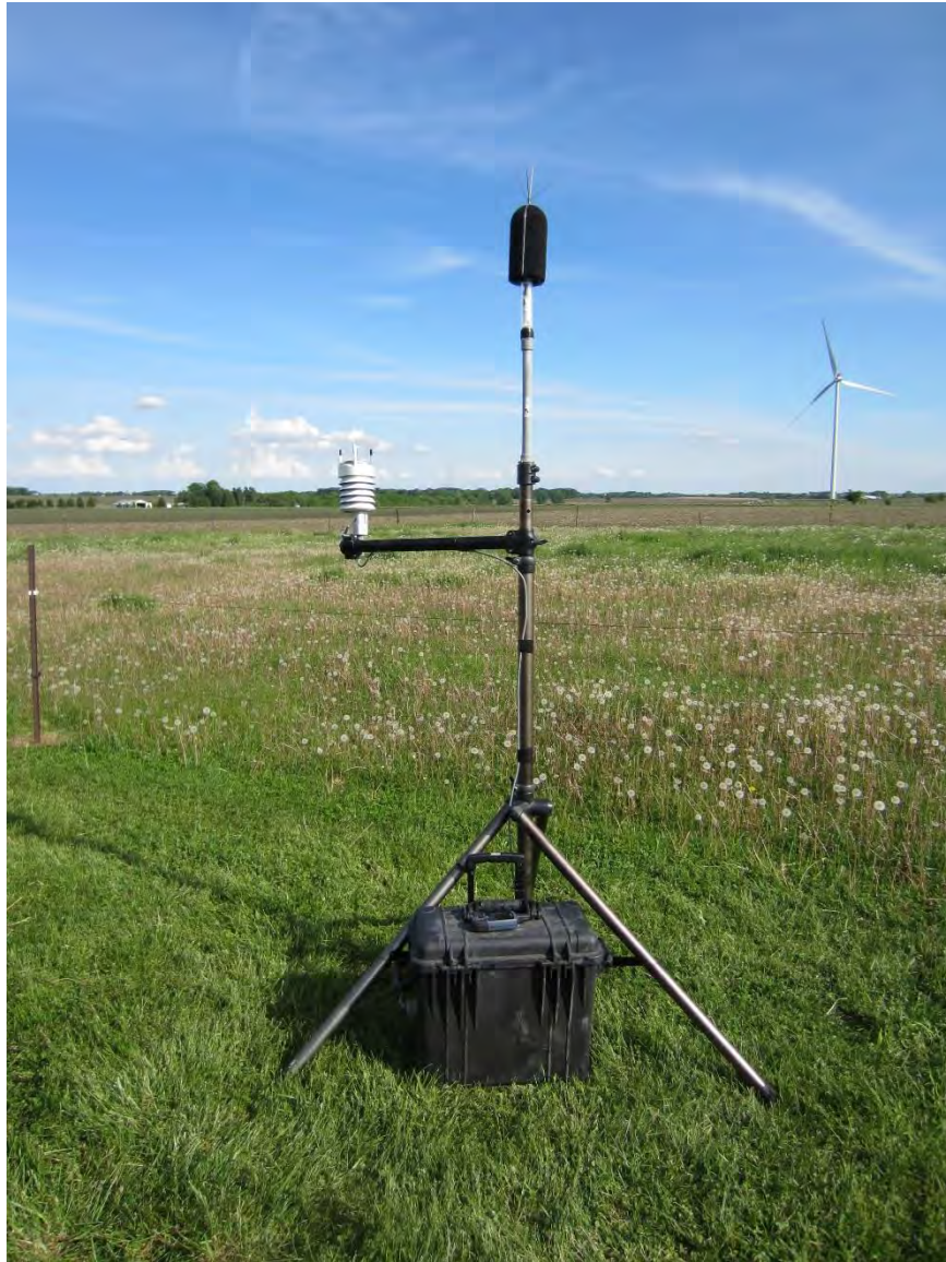
In-situ set-up of Sound Measurement Equipment
