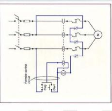
Exhibit 100.14 Remote-control circuit for starting and stopping
