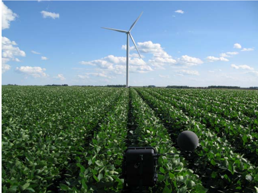
Figure 8 Field Sound Level Monitor 1000 ft. from a Typical Turbine with 175 mm Treated Windscreen
