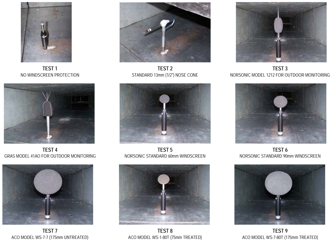
Figure 4 Test Windscreens as Mounted in Wind Tunnel
